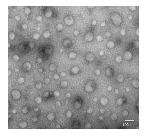
Transmission electron microscopy (TEM) micrography of exosomes recovered from NIH3T3 cell media with <u>PureExo® Exosome</u> <u>Isolation kit</u>.
